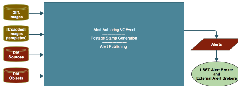
Figure 5: Illustration of the conceptual algorithm design for Image Differencing, Difference Image Analysis, and Alert Generation and Distribution pipelines.
