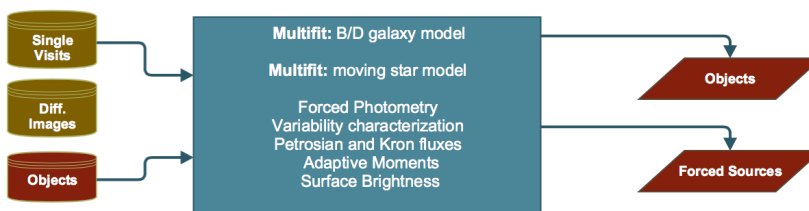
FIGURE 4: Illustration of the conceptual algorithm design for Image Coaddition, Coadded Image Analysis, and Multi-epoch Object Characterization pipelines.
